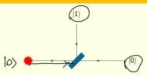
The beam-splitter sends a photon along a superposition of paths
