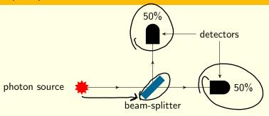
A system with two states can be built by placing photon detectors at two locations
